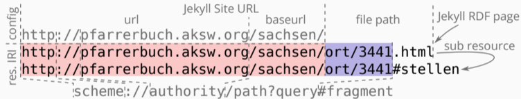
Figure 1: Scheme of the selection of page paths based on the configured Jekyll Site URL.
